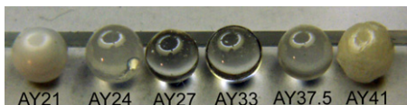
Figure 1. Photographs of \approx 2.3 – 2.5 mm diameter solid samples of (Y_2O_3)_x(Al_2O_3)_{1-x} produced on the aerodynamic levitator. The labels correspond to the following compositions: AY21 ( x = 0.21 ), AY24 ( x = 0.24 ), AY27 ( x = 0.27 ), AY33 ( x = 0.33 ), AY37.5 ( x = 0.375 ) and AY41 ( x = 0.41 ).
